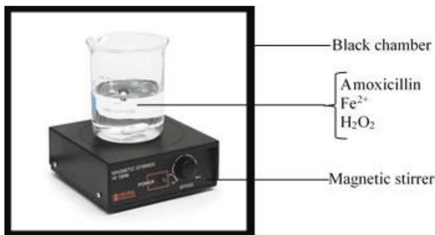
Fig. 2. Schematic representation of Fenton process
