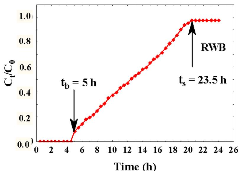
**Fig. 8. Breakthrough curve relating to the treatment of RWB**
