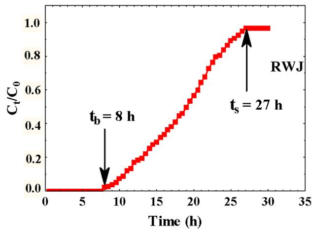
Fig. 7. Breakthrough curve relating to the treatment of RWJ
