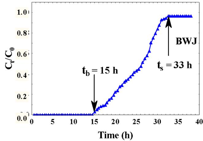
Fig. 6. Breakthrough curve relating to the treatment of BWJ
